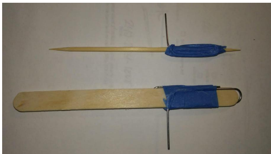
Figure 1b. Securing the wire to the core.
