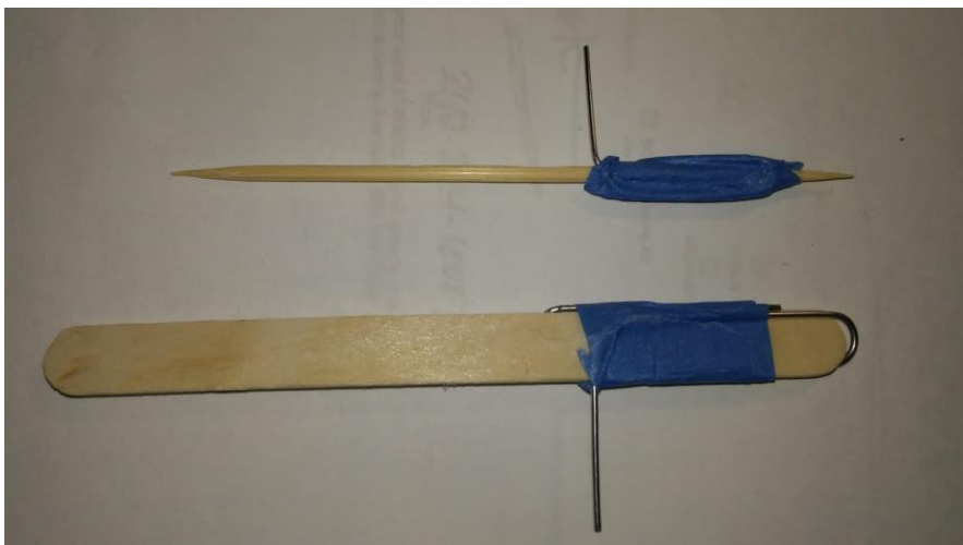
Figure 1b. Securing the wire to the core.
