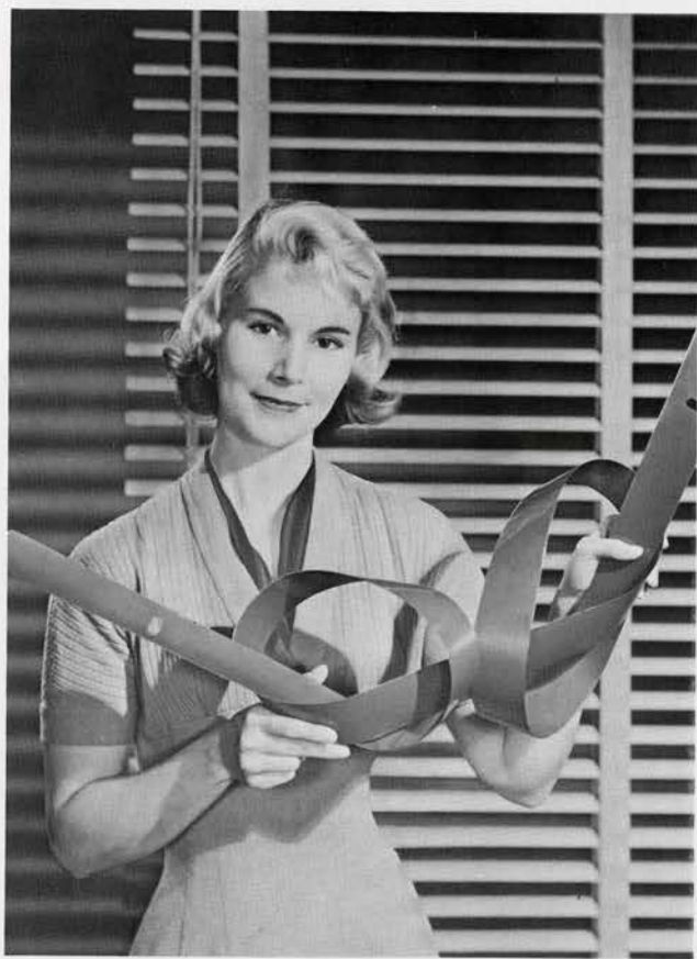
Tin mill blackplate is widely used in making venetian blinds, toys, and other light articles. Steel in this form is strong and flexible.
