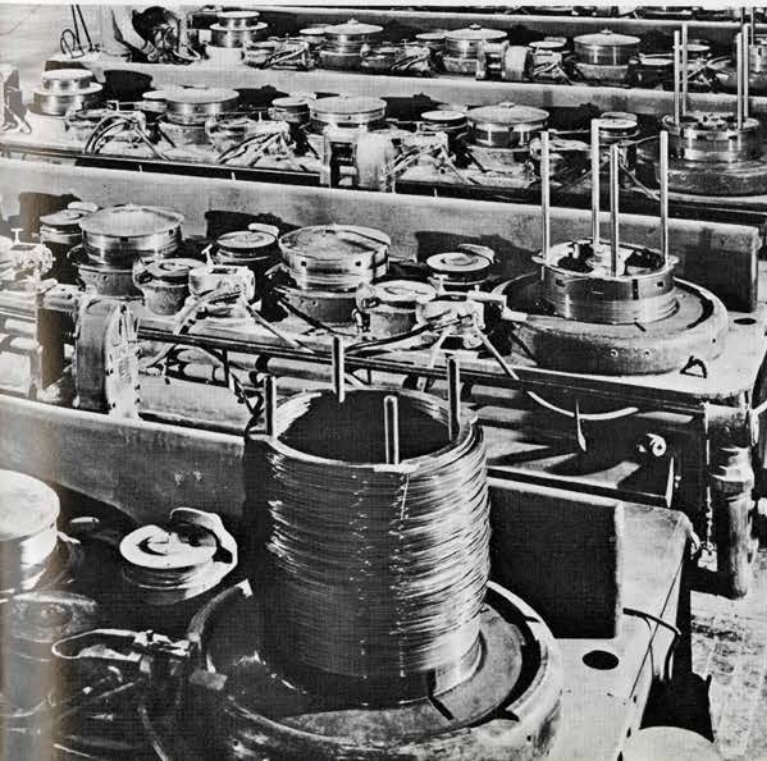
Battery of modern wire-drawing machines. Rod enters at the left, is reduced in size as it passes through successive dies, and is coiled.
