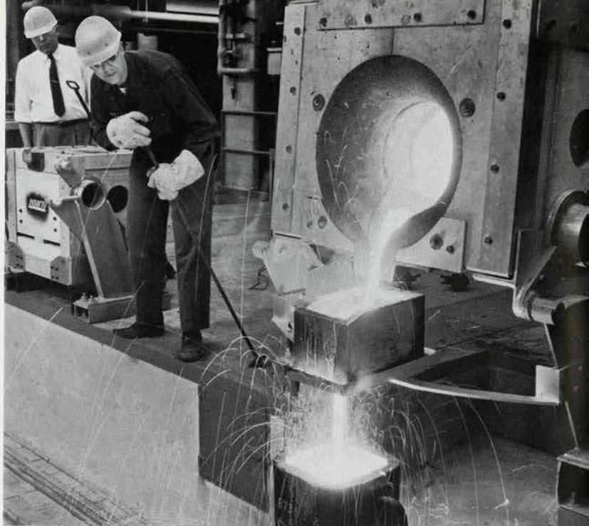
Pouring an experimental melt of 300 pounds of steel.
