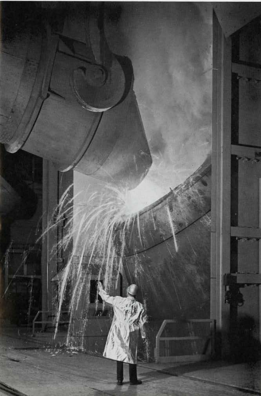
After a basic oxygen furnace is loaded with steel scrap, it is charged with molten iron. It takes about 5 minutes to do both.
