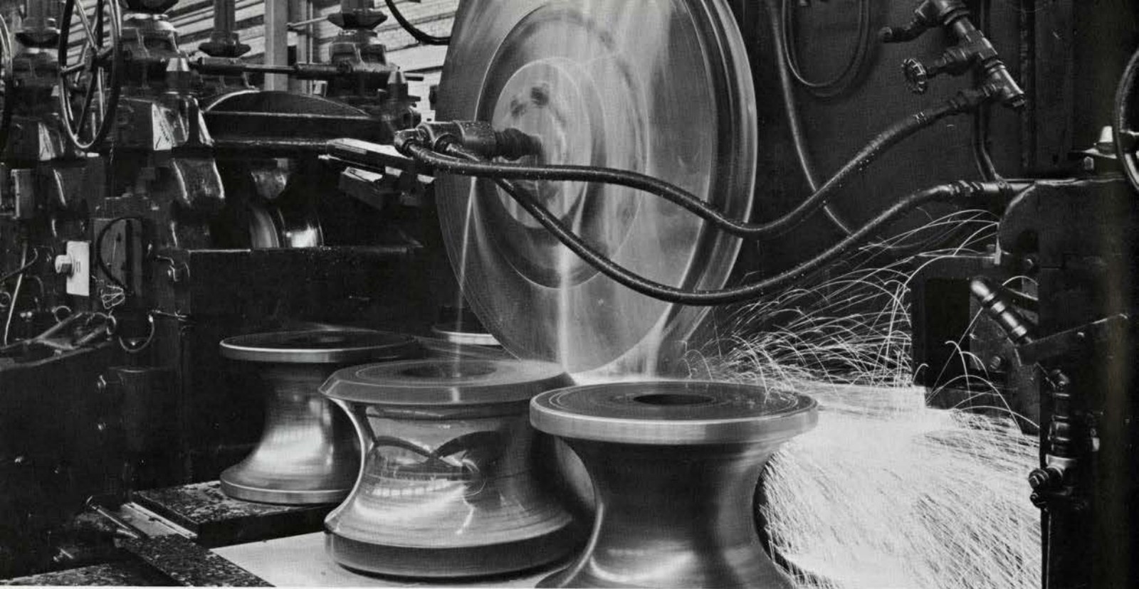
In the electric resistance-welding process, skelp from the forming rolls (left) is welded automatically.
