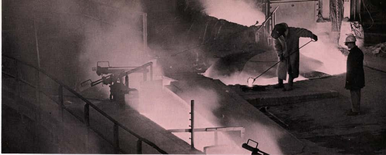
Blast furnaces operate continuously. Molten iron is tapped every five or six hours.
