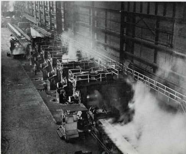
Sheet steel emerging from a continuous hot-sheet mill. In the background a partially reduced slab nears the finishing stands.
