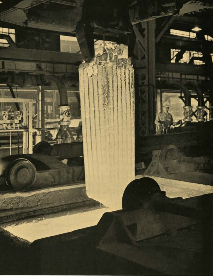
Powerful tongs lift an ingot from the soaking pit where it was thoroughly heated to the rolling temperature.
