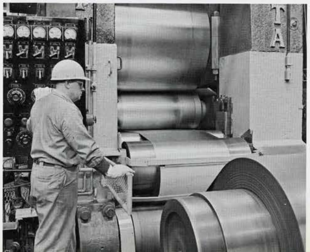
After cold rolling, steel is softened by annealing, then passed through this skin-pass mill which stiffens and polishes the steel.
