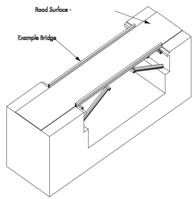
Orthogonal Sketch of Simple Bridge Shown Over Hazard Road bed must be at least 6"wide
