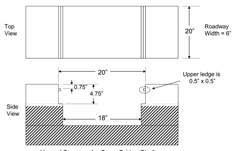
Hazard Structure for Straw Bridge Challenge. Do not support bridge from hatchmarked areas. Not to Scale
